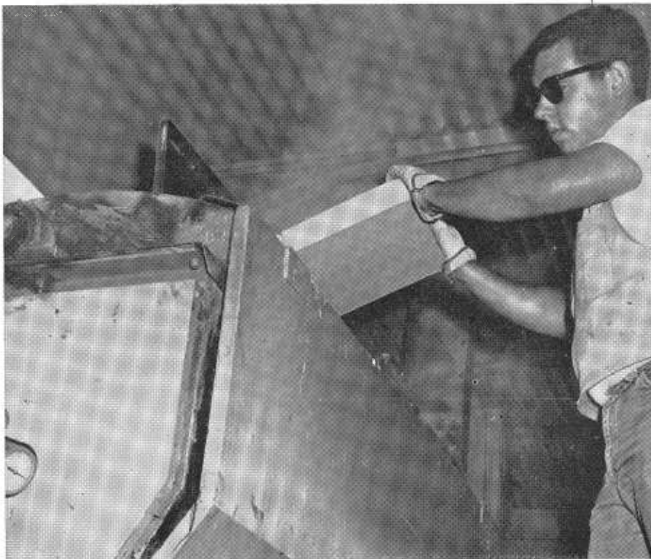
Charging the kettle with solid thermoplastic material. Repeated heating of the material does not harm it.
