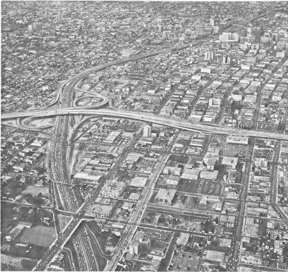
URBAN—The heavily traveled Harbor Freeway in Los Angeles, running from top to bottom in this photo, is an example of a Federal-Aid highway on the Primary system within an urban area. The interchange at left center connects it with the Santa Monica Freeway, which is on the Interstate System.
