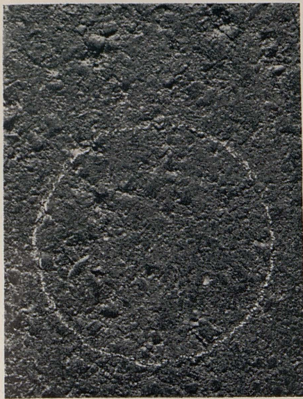
FIGURE 4A. Relation of permeability to surface texture. Penetration rate on this section was 10 millimeters per minute.
