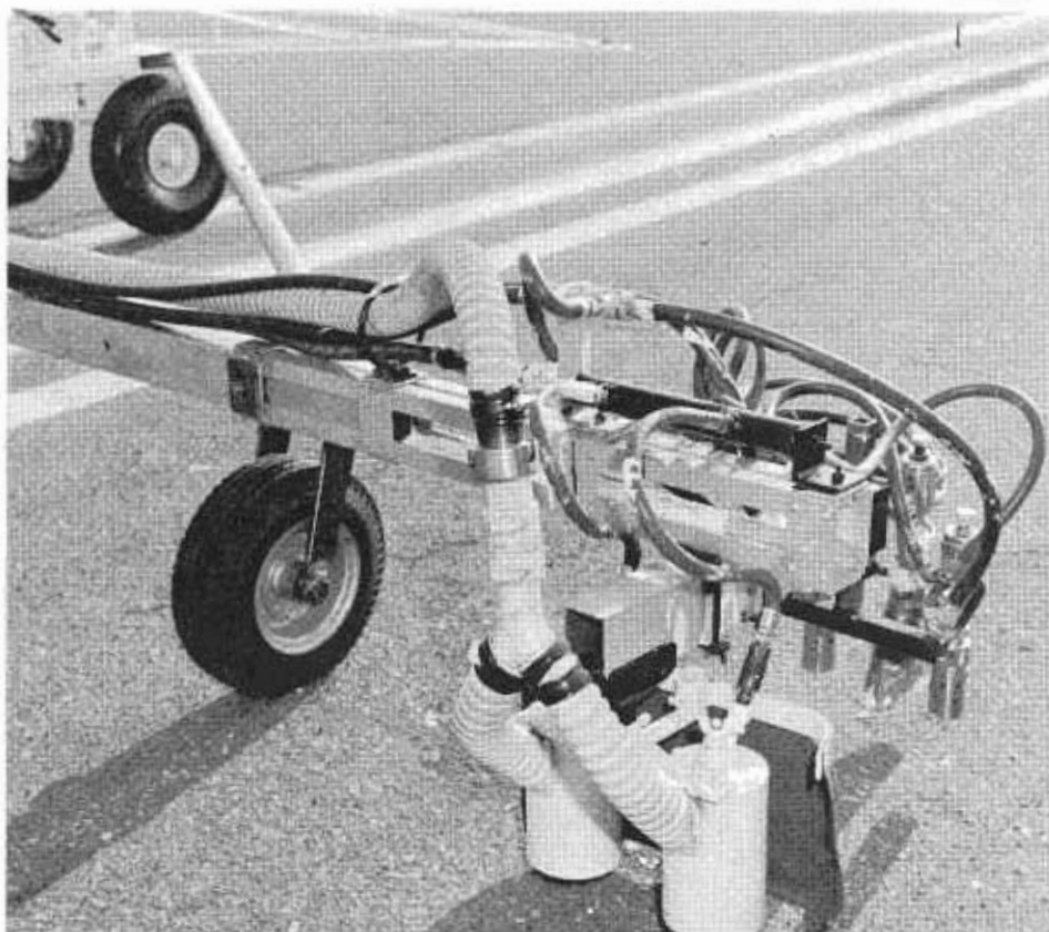
Paint guns and bead dispensers on the end of the lightweight extension arm.
