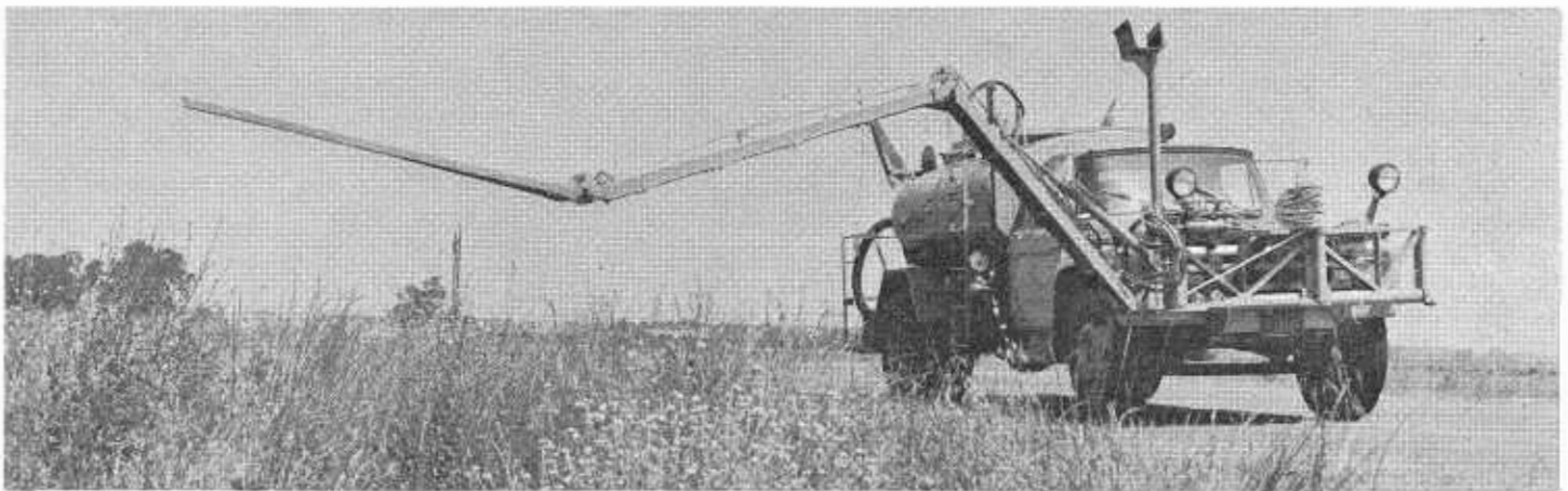
This combination water tanker and roadside spray unit with cab-operated hydraulic spray boom is used for applying liquid fertilizers or soil sterilants.
