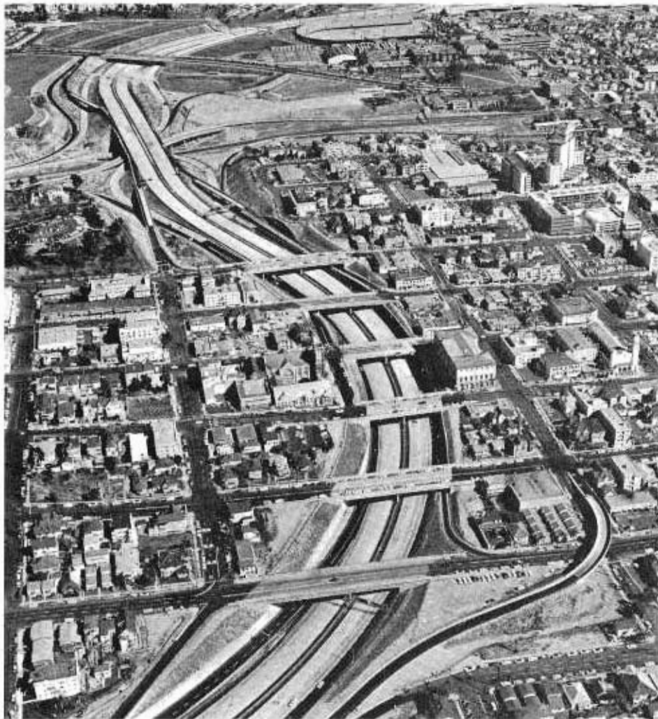
The Interstate 5 Freeway looking east from the north edge of San Diego's business district. Canyon reclaimed by highway embankment is discernible in left background.
