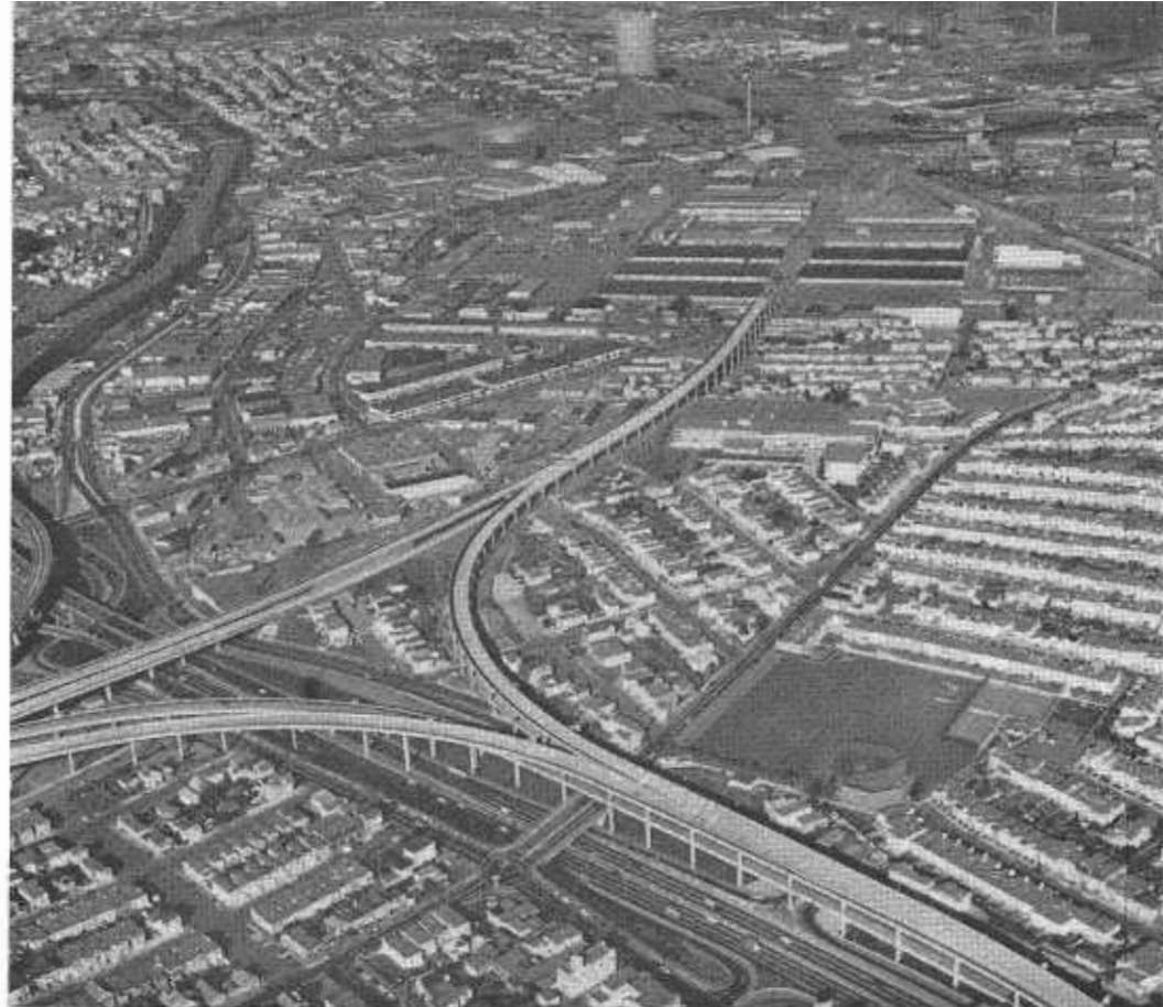
The Route 82 Freeway in San Francisco extends northeasterly across the US 101 (James Lick Memorial) Freeway as a two-level structure to the vicinity of a future interchange with the adopted freeway routing via Hunters Point. The new budget provides funds to extend it northerly as the Route 87 Freeway to north of 18th Street.
