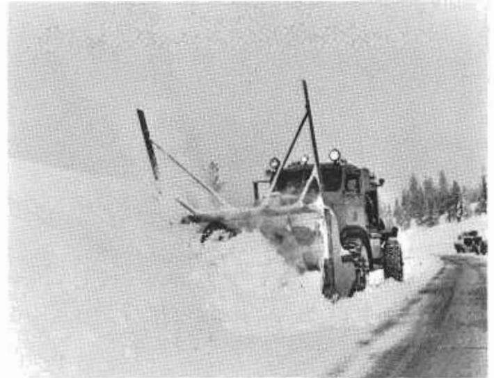
"Sno Blo" was redesigned and rebuilt at Headquarters Shop. It has approximately double the capacity of the old rotary plow.
