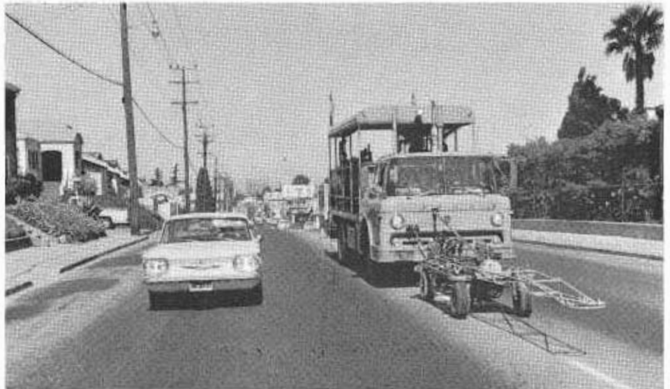
The new model traffic striper is shown in operation in Oakland.
