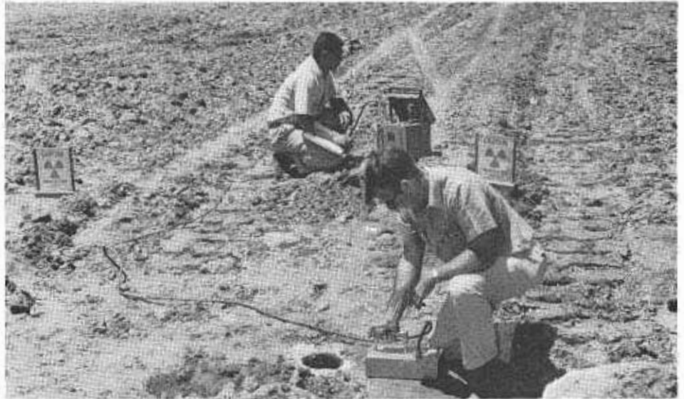
Technicians use nuclear moisture density gauges in field comparisons with conventional methods.
