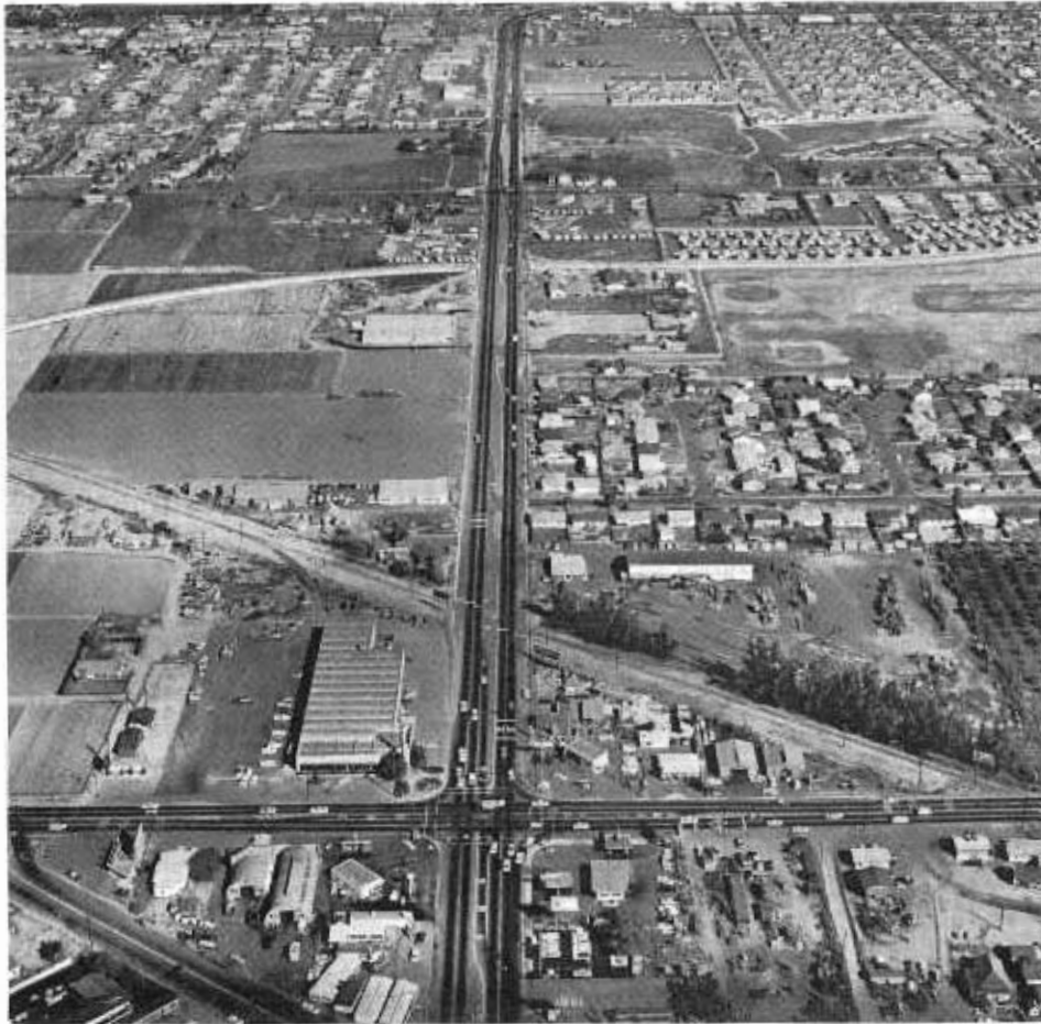
The southern end of the Harbor Boulevard reconstruction looking north. The future Garden Grove Freeway will cross near the upper part of the photo. The openings and left turn pockets in the center strip were provided for present and future improvements (shopping centers and streets).
