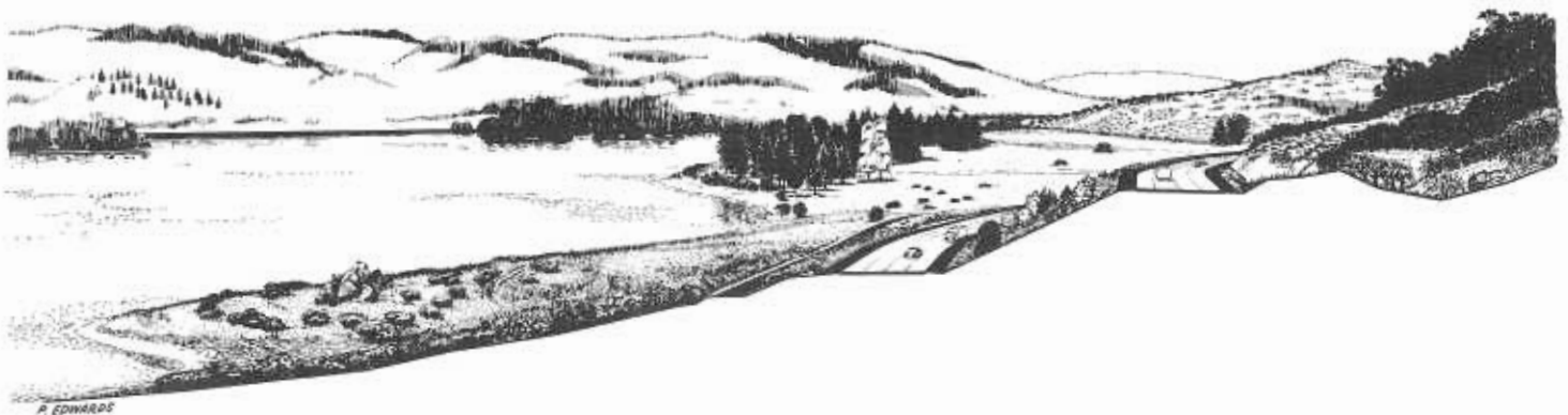
Drawing of a section of Interstate 280 (looking north) showing the split-level independent roadways for each direction of travel passing through scenic vistas surrounding the Crystal Springs Reservoir. The area shown above is just south of the site of the future San Mateo Creek Bridge.
