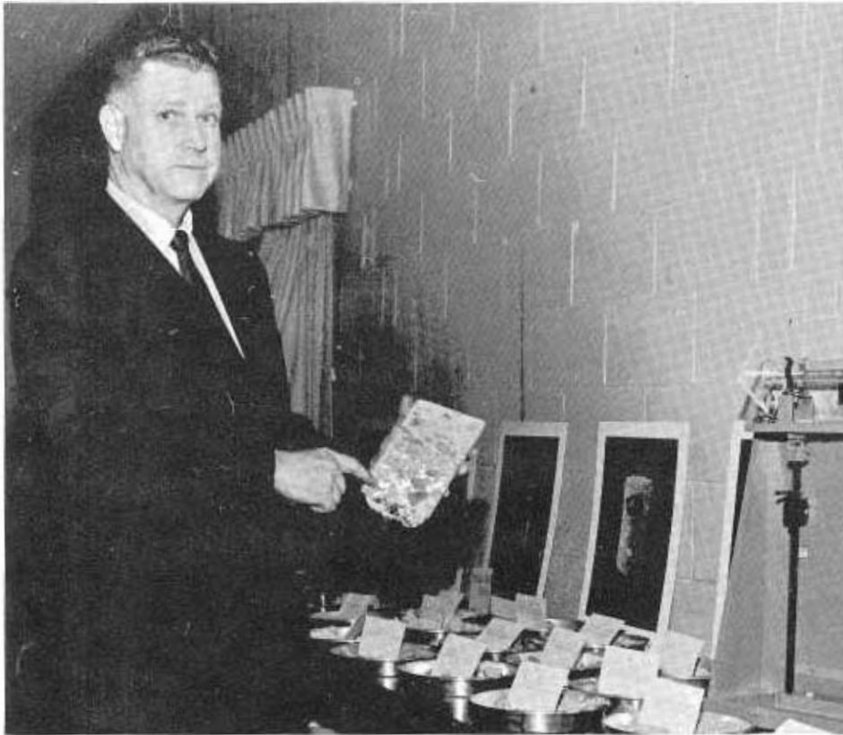
Leigh Spickelmire, Headquarters Construction, holding a test core. The exhibit table contains an Idaho Sand Shaker and aggregate samples used in conducting small group lectures.
