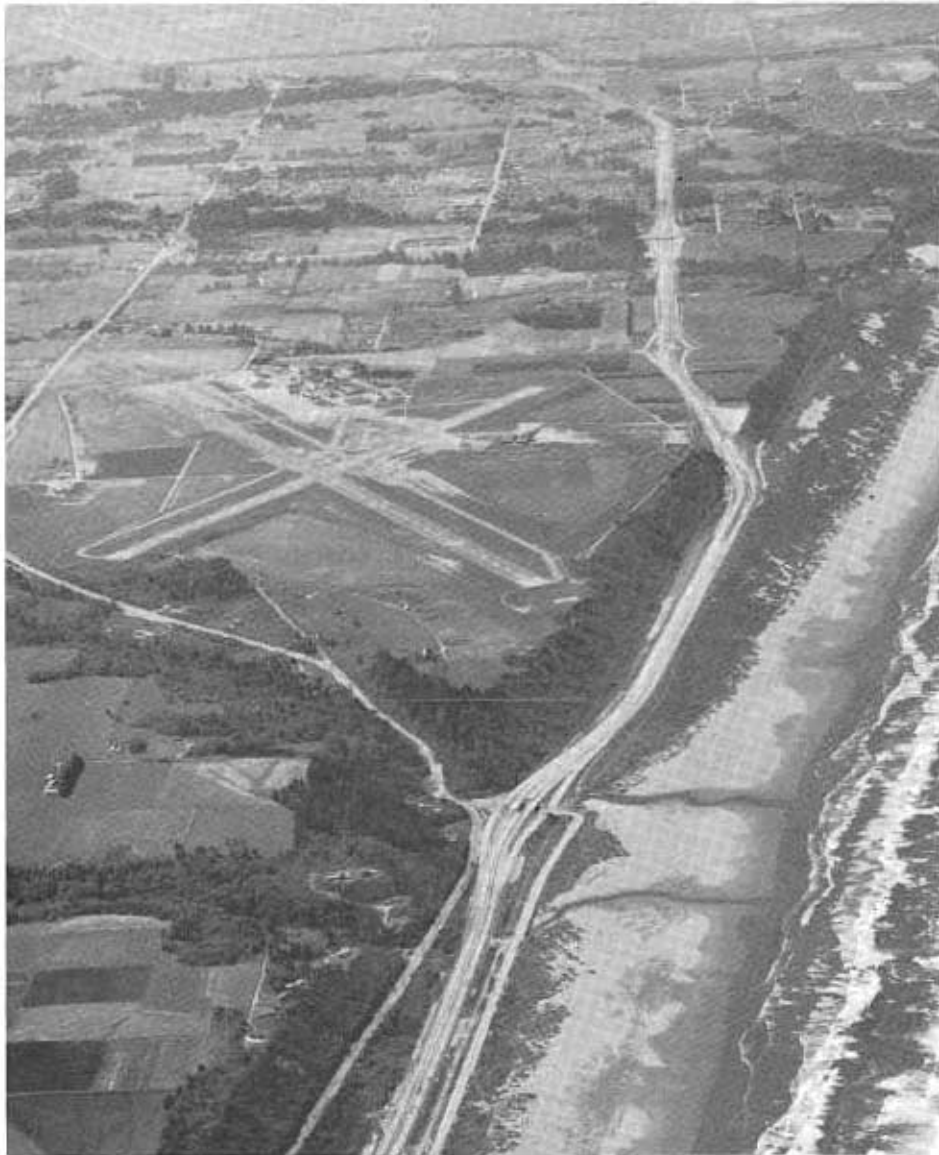
An aerial of the McKinleyville Freeway looking south. Clam Beach Interchange is in the foreground. The old highway through McKinleyville is to the left and Arcata Airport center. Frontage road right of freeway in foreground provides parking for 350 cars and unrestricted access to the beach for 1½ miles. Photo by David Swanlund.
