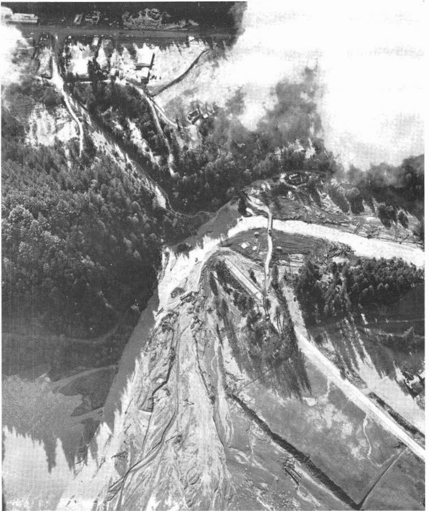
View from air of break at Willow Creek Bridge on State Route 96, emergency log bridge and collapsed bridge in center. Trinity River at lower left, town of Willow Creek and Route 299 top of picture.
