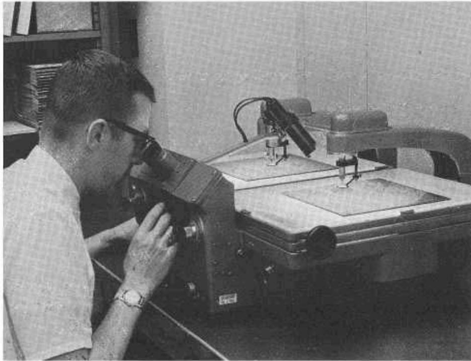
This point transfer device is a precision stereoscopic instrument used in the operation of photogrammetric control bridging.
