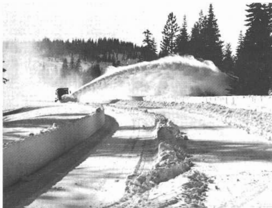
One of the yearly tasks of maintenance crews is snow removal from state highways. Here, a rotary snowplow removes snow from a section of Interstate 80 in the Donner Summit area.
