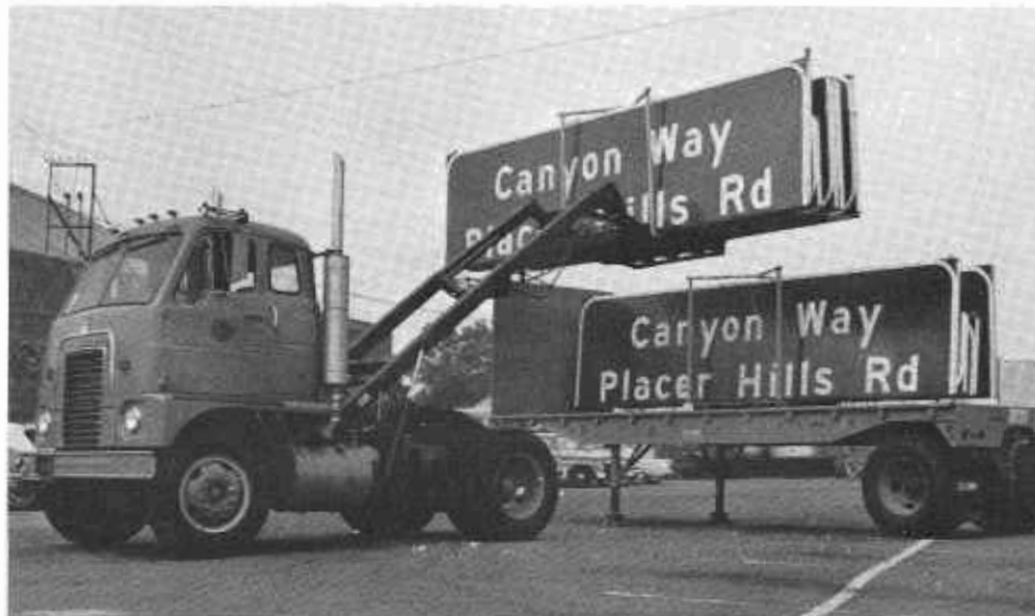
Among the new pieces of equipment purchased by the Division of Highways is this new forklift truck shown loading freeway signs on to a trailer.
