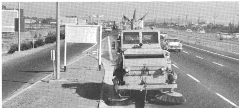
A rotary sweeper cleans gutters on the Bayshore Freeway in San Mateo County south of San Francisco.
