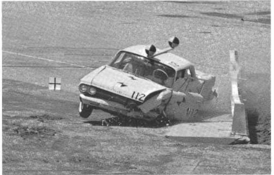
Full-scale dynamic impact tests such as that shown in this photo are conducted by the Division of Highways to test design of bridge rails and median barriers.
