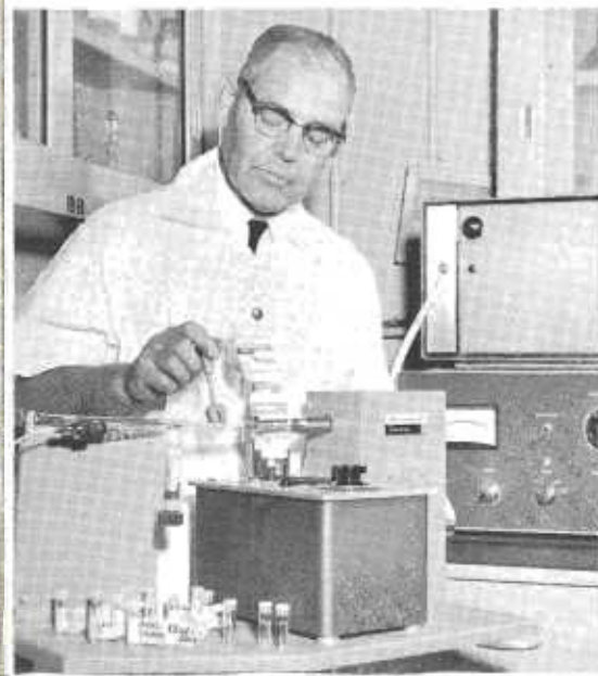
PHOTO ABOVE—An engineer checks data being received from a recorder inside a trailer at a jobsite. The trailer contains all the receiving and recording equipment for collecting information transmitted by strain gages used in a research study of an orthotropic bridge constructed near Dublin in Alameda County. BELOW—a chemical engineer uses a gas chromatograph to determine the constituents of paints and solvents.
