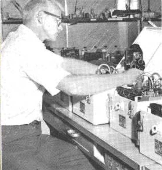
An engineer installs a motion picture camera into its control box for gathering data on wrong-way drivers as part of a safety study.
