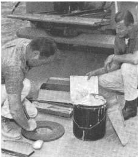
In-place densities of compacted roadway material is determined by measuring weight and volume of material removed from a carefully excavated hole.
