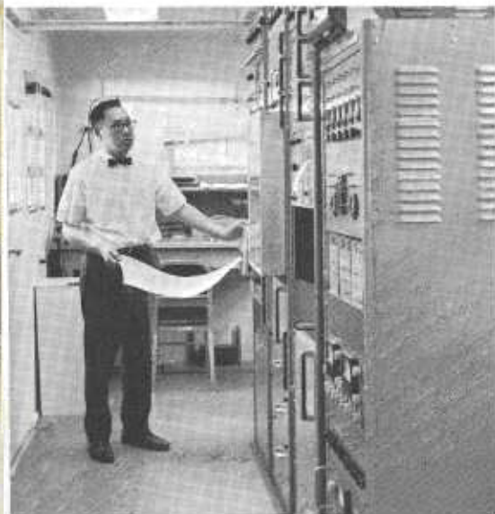
PHOTO ABOVE—An engineer checks data being received from a recorder inside a trailer at a jobsite. The trailer contains all the receiving and recording equipment for collecting information transmitted by strain gages used in a research study of an orthotropic bridge constructed near Dublin in Alameda County. BELOW—a chemical engineer uses a gas chromatograph to determine the constituents of paints and solvents.
