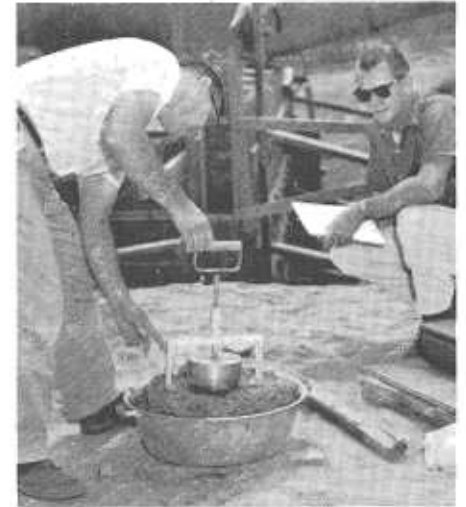
A construction inspector teaches a trainee in the proper determination of concrete slump with the Kelly-ball device.
