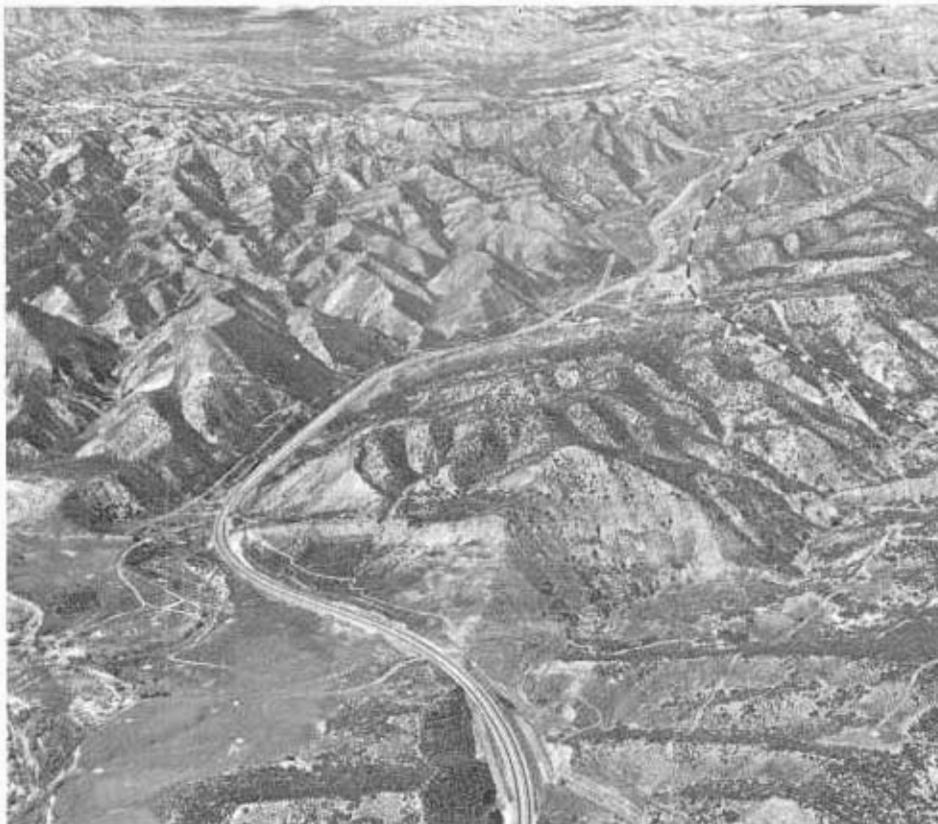
Looking north from Liebre Gulch along the existing Ridge Route with the projected new route indicated by the broken line (upper right).
