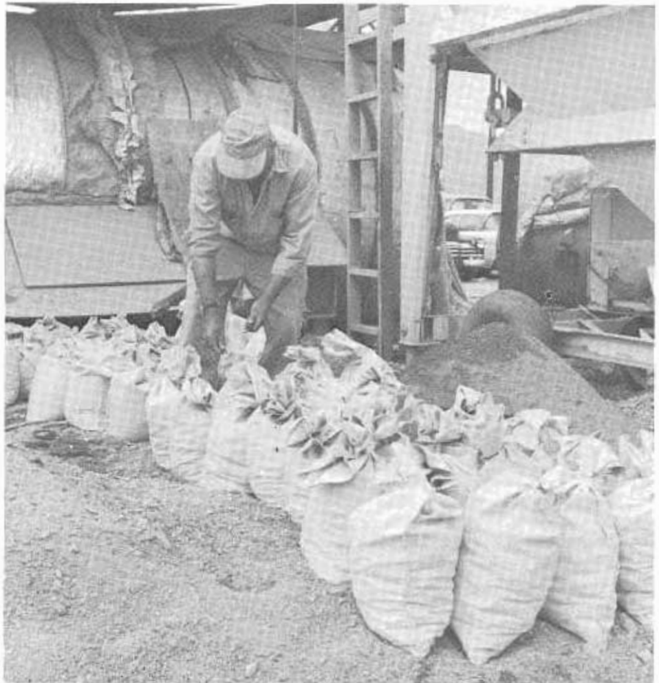
Norman Schmutz of the Bridge Department prepares concrete aggregate samples for shipment to the District Laboratory. Samples shown represent approximately 1,200 tons of aggregate.
