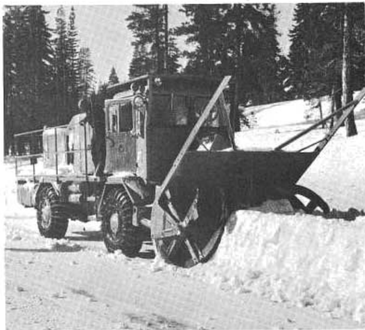
This 19-ton rotary plow is used in areas of combined heavy snow and high traffic volume, such as Interstate 80 in the high Sierra.
