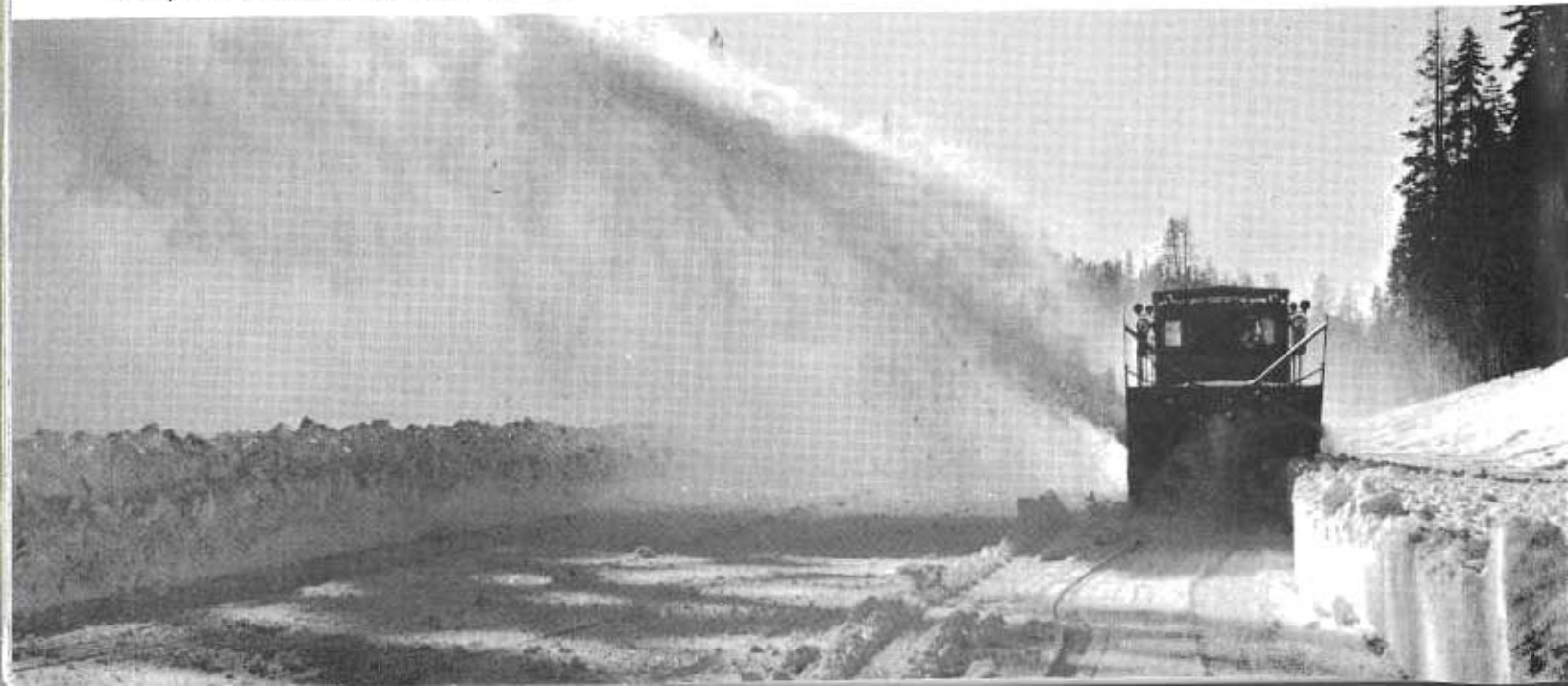
This machine, same as above, can throw up to 2,200 tons of snow per hour. Power comes from two diesel engines (220 horsepower for propulsion and 335 horsepower for feeder and rotary blades).
