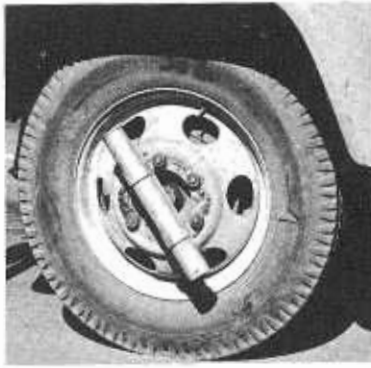
Automatic snow stake driver was invented by District 9. Mechanism on front left wheel determined when next pole should be plunged earthward by the hydraulic rig. Workmen place one stake every 50 seconds for a daily total of 600.
