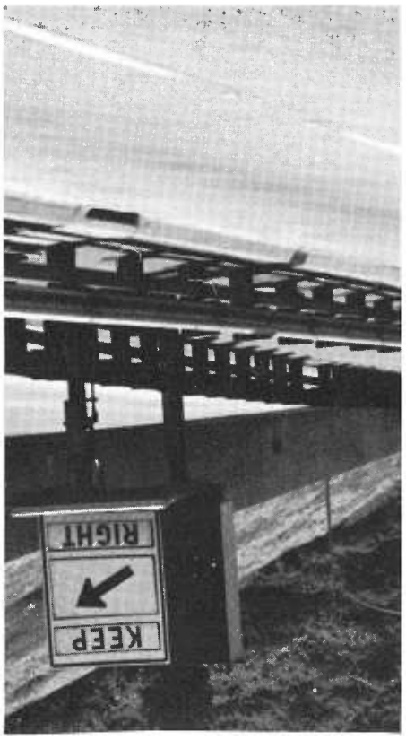
MESSAGING CHANGE. In the photo sequence above a button flips message prisms in a sign changing double arrows to single arrow and "keep right."
