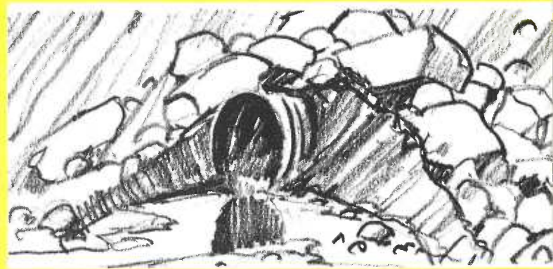
Structures to protect culvert openings are usually not necessary. Piled rocks will do as well in most cases, and are much less noticeable.
