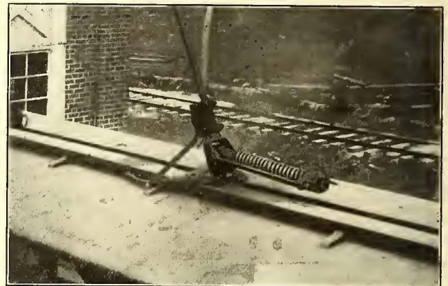
Pole Clamp Loose So That Pole May Be Removed
