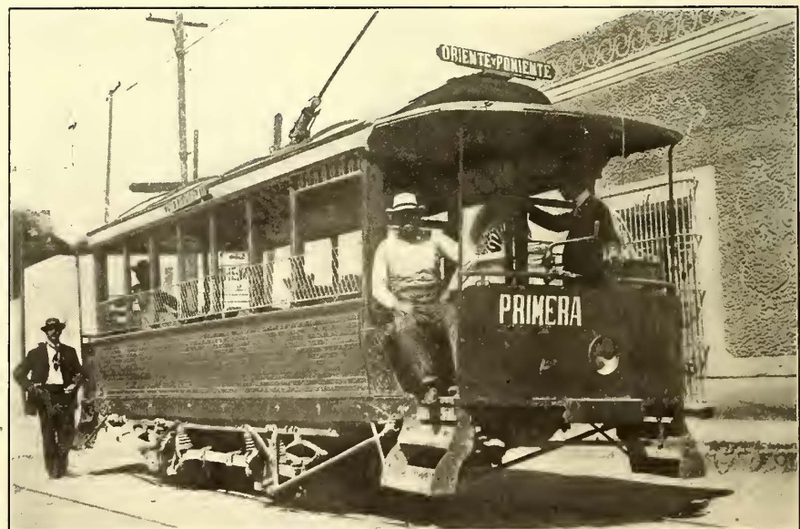
Single-Truck Car for City Service
