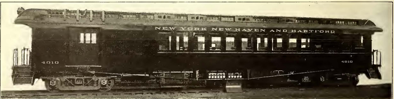
Combination Passenger and Baggage Car for the Electrified Branch of the New York, New Haven & Hartford Railroad Between New Canaan and Stamford
