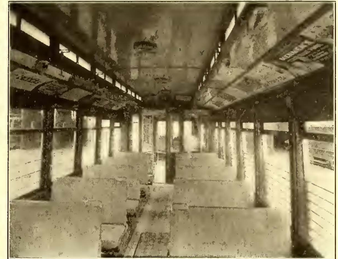
Passenger Section of Side Entrance Pay-as-You-Enter Car motors, was built at the Montreal Street Railway Company's shops, Hochelaga, at a cost of $11,000. The car body alone cost from $4,000 to $5,000.
