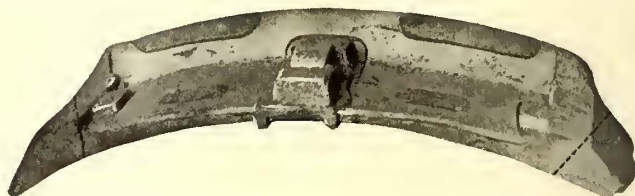
Fig. 16.—Worn Subway Shoe, 1907 Type, Dotted Lines Showing Where Toes Have Been Cut Off to Reduce the Scrap 4 Lb. Per Shoe
