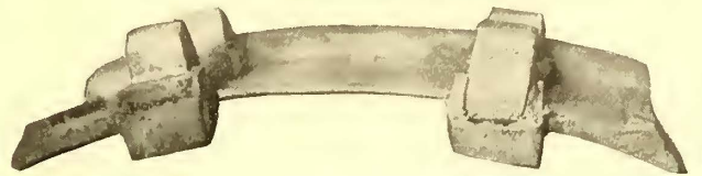
Fig. 8.—Worn Manhattan Motor Shoe, Shown New in Fig. 4
