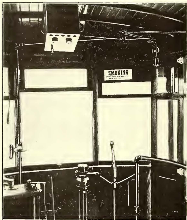
St. Louis Pay-as-You-Enter Car—Door Operating Mechanism at Front End
