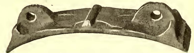
Fig. 10.—Manhattan Trailer Shoe, Scrap Weight 10 1/2 Lb., 60 Per Cent Wear
