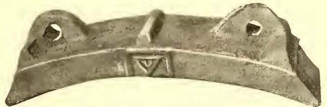
Fig. 9.—Manhattan Trailer Shoe, Weight 27 Lb. Net, 60 Per Cent Wear
