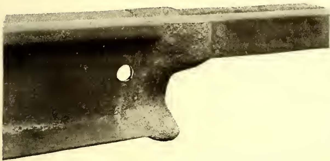
Compromise Weld of Deep and Shallow Rail Made for Central Bridge of the Union Railway Company
