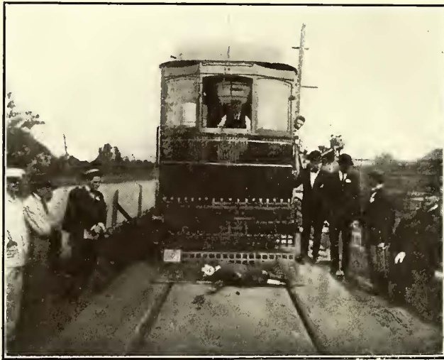
Public Service Commission Fender Tests at Schenectady—Two Successful Pick-ups of a 50-lb Dummy on Smooth Pavement by a Grid Fender with Automatic Trippers
