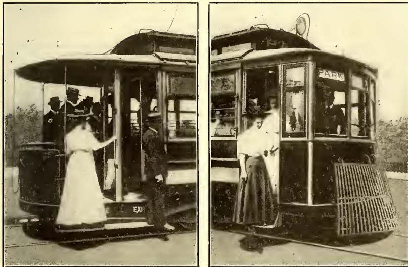
Rear and Front Platforms of Pay-As-You-Enter Cars St. Louis, Showing Bulkheads on Platform
