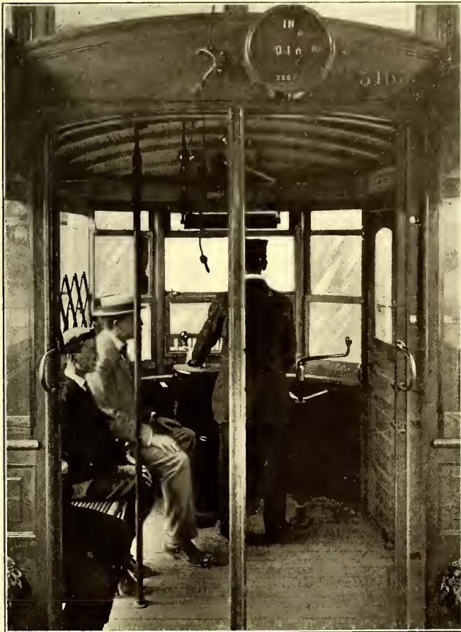
Metropolitan Standard Car—Front Platform, Showing Folding Seat for Passengers
