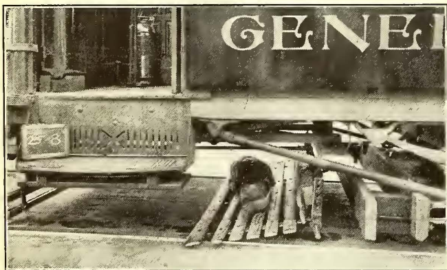
Fig. 4—Wheel Guard Applied to Test Car at Schenectady, Showing Tray Lowered
