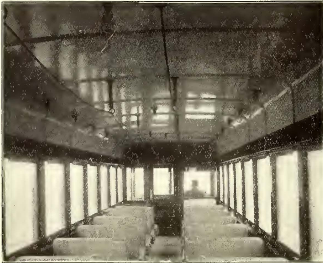
The Barber Car in Sunbury, Pa.—Interior, Showing the High Windows, Lighting Arrangement, Body, End Door, Etc.
