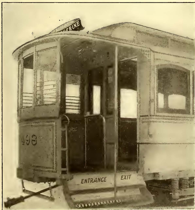
Rear Platform of Rebuilt Montreal Single-Truck Car
