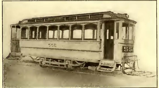
Montreal Single-Truck Car as Rebuilt for Pay-As-You-Enter Service
