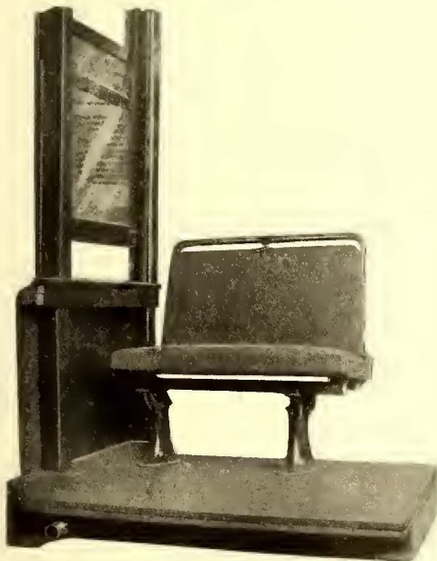
St. Louis Steel Car—Leg Space Between Posts
