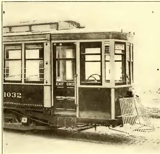
St. Louis Steel Car—Front End, Showing Fuse-Box on Vestibule Corner Post
