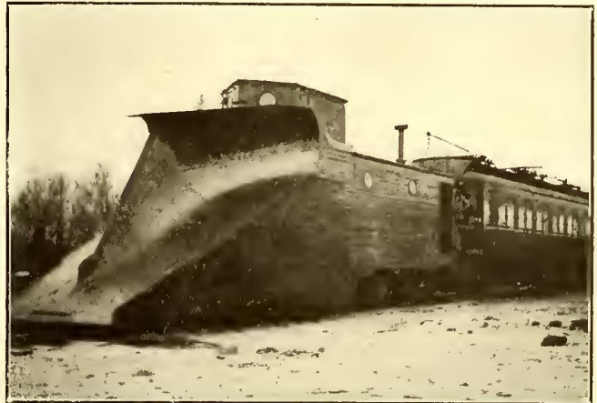
Chicago, Lake Shore & South Bend—Russell Snow Plow Pushed by Standard Passenger Car
