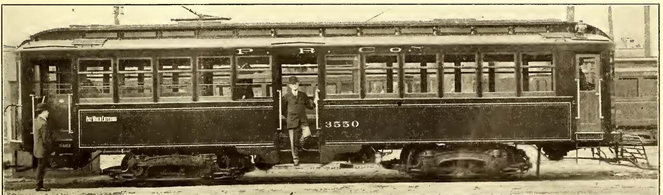
Pittsburg Corridor Prepayment Car—Entering at the Rear and Leaving at the Center
