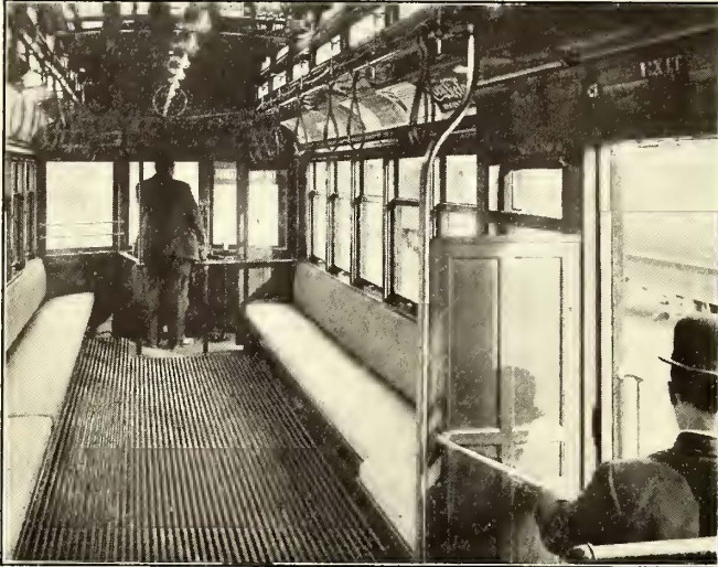
Pittsburg Corridor Prepayment Car—Illustrating the Positions of the Motorman and a Departing Passenger
