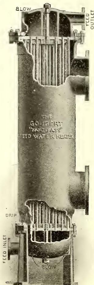
Closed Feed-Water Heater
