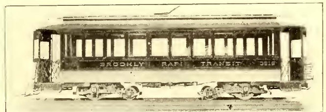
Fig. 9—Brooklyn Rolling Stock—Semi-Convertible Car, with Maximum Traction Trucks, 3500 Type
