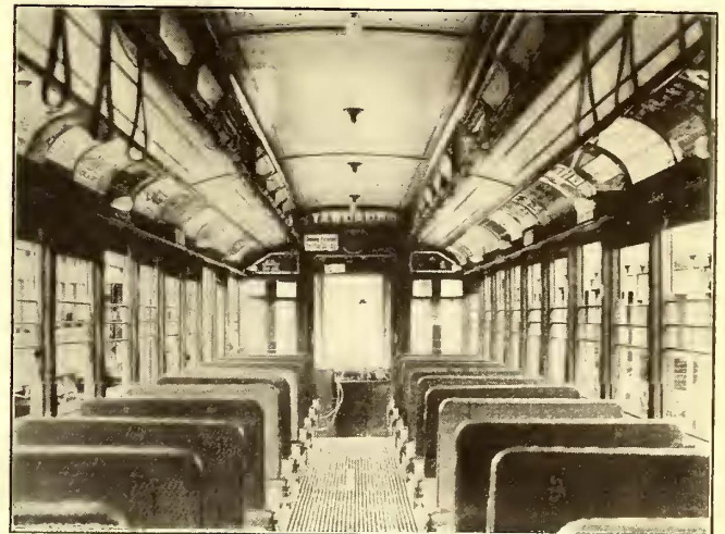
Fig. 9—Brooklyn Car Lighting—Interior of Convertible Surface Car
