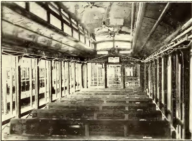
Fig. 10—Brooklyn Car Lighting—Center Lamps in Double-Track Open Car
