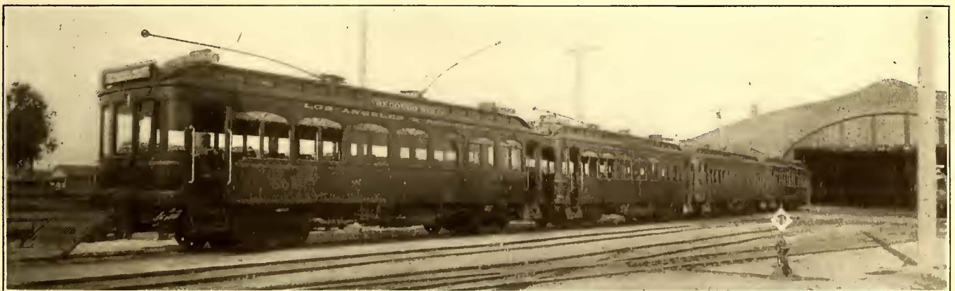
Los Angeles & Redondo Railway—Multiple-Unit Train Built in Company's Shops and Regularly Operated in Service to Redondo Beach
