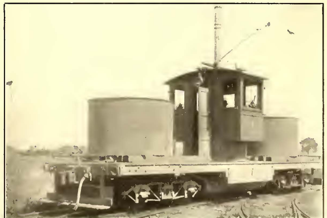
Central California Traction—Combination Work Car and Sprinkler
