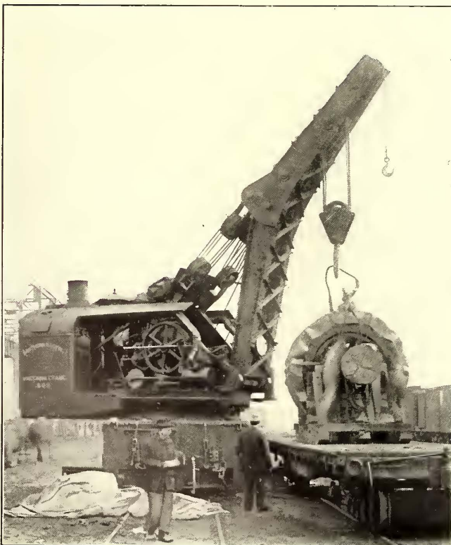
United Railroads of San Francisco—Handling Electrical Machinery with Wrecking Crane
