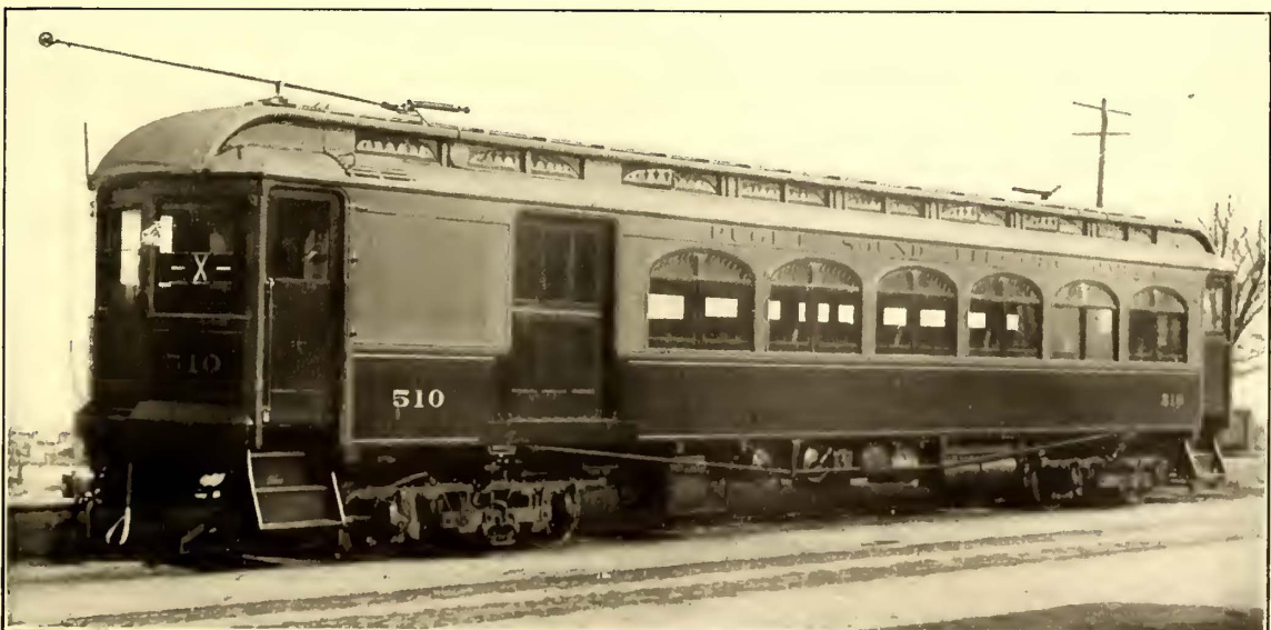
Puget Sound Electric Railway—Combination Baggage and Smoker Motor Car
