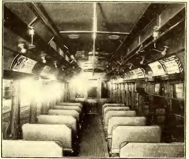
Interior of Chicago Car, Showing Exhaust Ventilators in Ceiling
