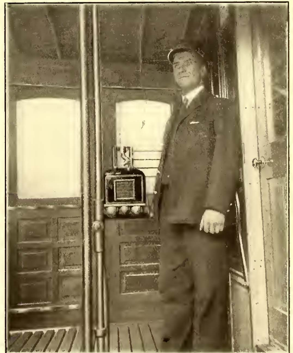
Fare Box Mounted on Car Platform
