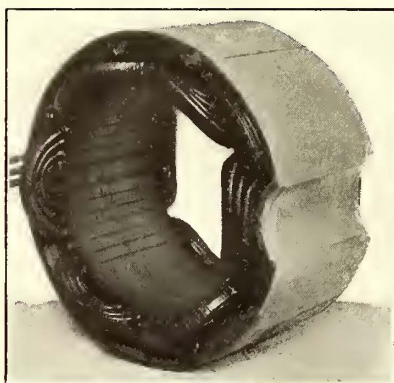
Hamburg-Blankenese-Ohlsdorf Railway Improvements—Stator and Rotor of New Single- Phase Motor
