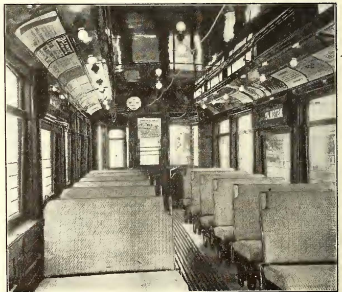
Chicago Railways Car Reconstruction—Interior of Rebuilt Car, Showing Electric Lighting
