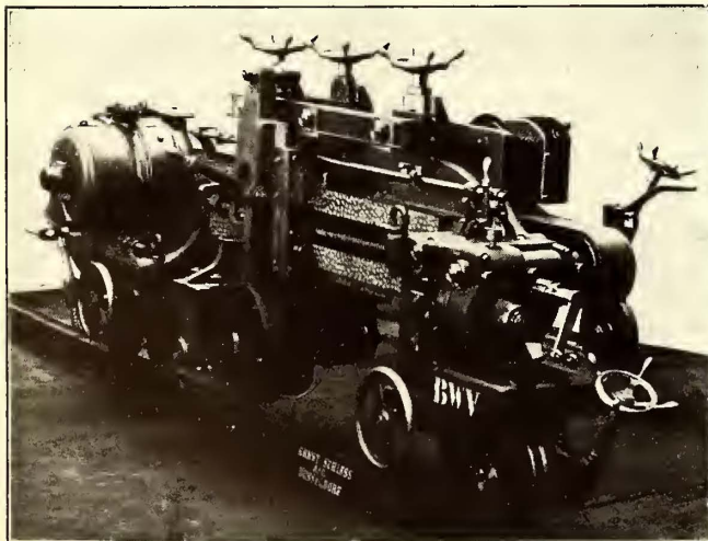
Fig. 2—Berlin Rail Welding—Emery Grinder
