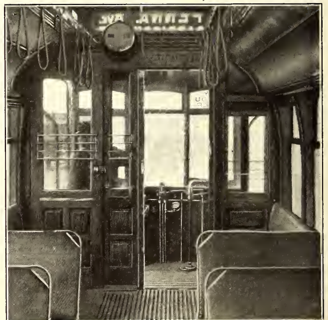
Baltimore Pay-As-You-Enter Cars—Door Arrangement in End Bulkheads
