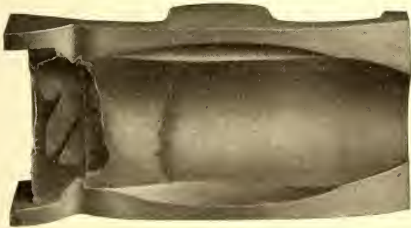
Composite Journal Bearing After a Run of 124,000 Miles
