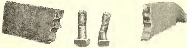
A Broken Motor Suspension Bar Which Was Responsible for An Accident
