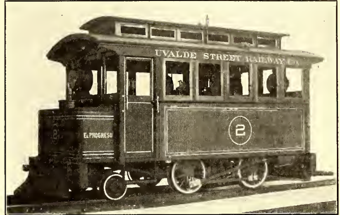
Enclosed Steam Locomotive for Street Service
