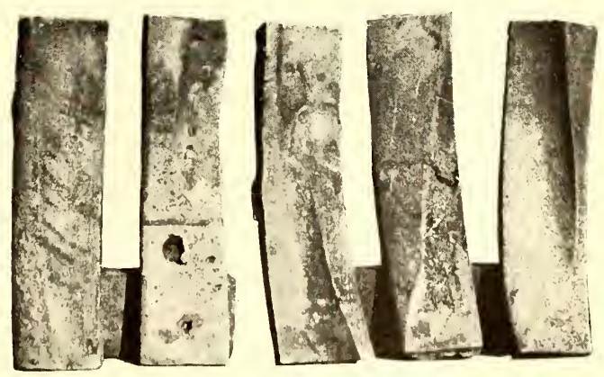
The Result of Improper Brake-Shoe Adjustment
