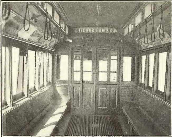
Metropolitan Rolling Stock and Shops—Double-Piece Door as Used in Converted Car and 1908 Prepayment Car
