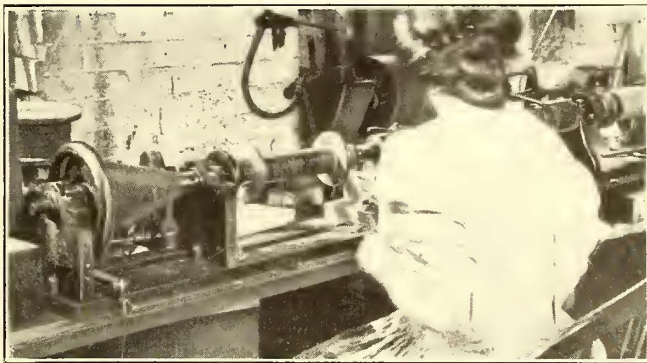
Fig. 10—Boston Elevated Shops—Winding Machine for Track Switch and Other Coils
