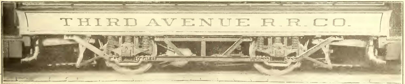
Truck and Chain Drive for the Motors of the Storage Battery Car
