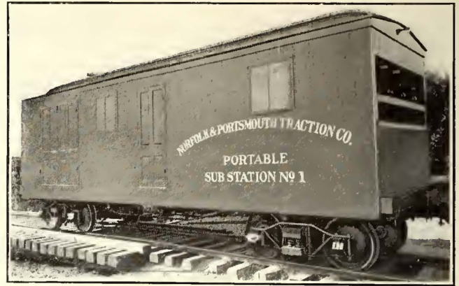
Norfolk Portable Substation—High-Tension End
