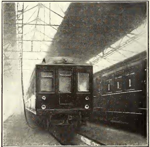
London Underground Railways—Flexible Overhead Connection for Moving Cars in Shed
