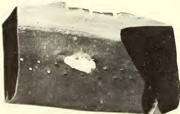
Fig. 11—Track Maintenance—Worn-out Soft Steel Conveyor Bucket
