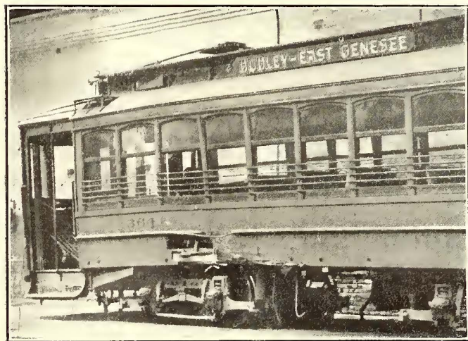
Car Struck by a Freight Train
