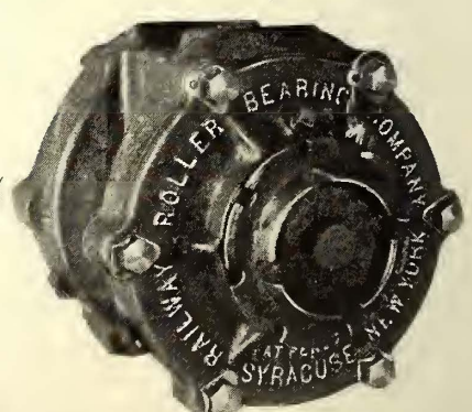
Philadelphia Anti-Friction Bearing Tests—Wiring Diagram of Test Car No. 2140 and View of Roller Bearing Encased
