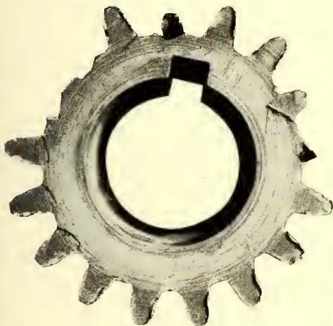
Pinion Failures—Fig. 1—Appearance of Tooth Fractures
